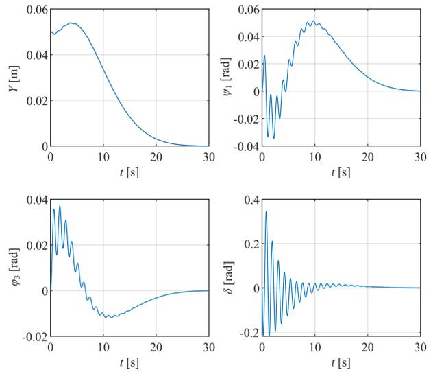
Fig. 4 Simulation results for the most stable gain-configuration (point  $S_1$ ). Control gains:  $P_Y = 5$  rad/m,  $P_{\psi_1} = -6.421$ ,  $P_{\varphi_3} = -13.82$ . Initial condition:  $Y(t=0) = 0.05$  m
