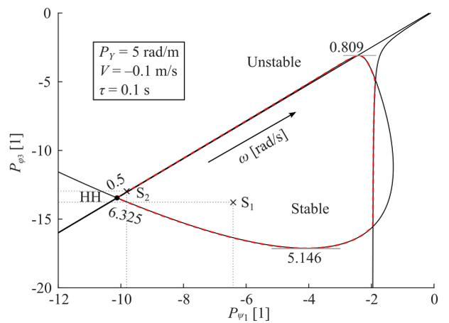
Fig. 3 Stability chart in the plane of control gains  $P_{\psi_1}$  and  $P_{\varphi_3}$  using both the D-subdivision (black continuous line) and the semi-discretization method (red dashed line).
