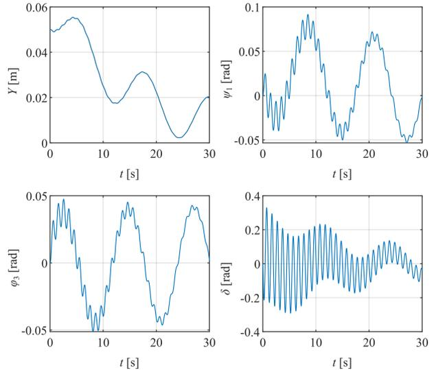
Fig. 5 Simulation results for a gain-configuration (point  $S_2$ ) picked from near the double-Hopf bifurcation point. Control gains:  $P_Y = 5$  rad/m,  $P_{\psi_1} = -9.8$ ,  $P_{\varphi_3} = -13$ . Initial condition:  $Y(t=0) = 0.05$  m
