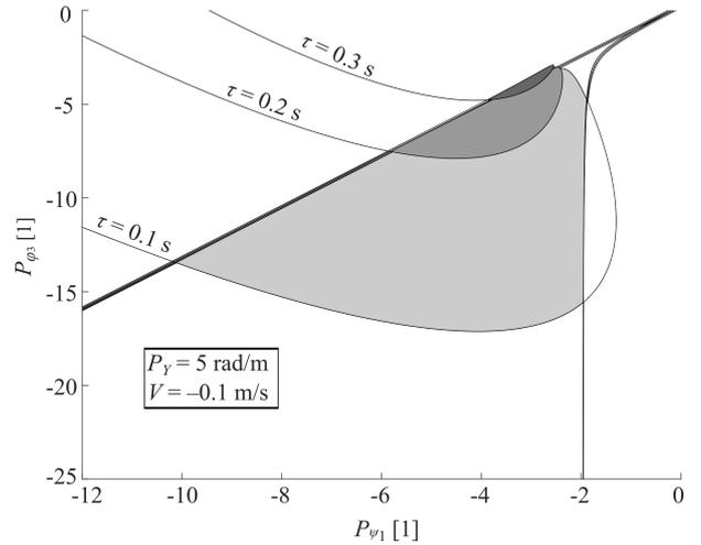
Fig. 2 Effect of time delay on stability. Different shades of gray relate to different value of time delay.
