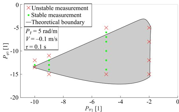
Fig. 7 Comparison of theoretical and experimental results: linear stability boundary (black curve) in the plane of control gains  $P_{\psi_1}$  and  $P_{\phi_3}$  for the parameters of the small-scale experimental rig (grey domain), and the measurement results (green dots and red crosses)
